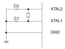
The Low Power Oscillator can operate in three different modes, each optimized for a specific frequency range. The operating mode is selected by the fuses CKSEL3:1 as shown in Table 10-3 on page 42.
