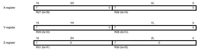
In the different addressing modes these address registers have functions as fixed displacement, automatic increment, and automatic decrement (see the "Instruction Set Summary" on page 404 for details).
