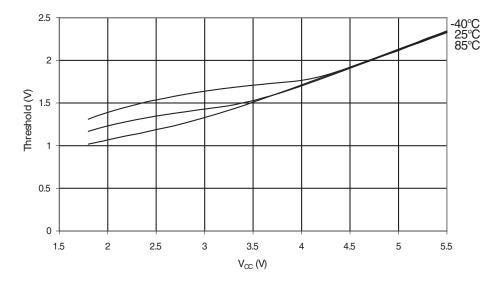
Figure 32-30. Reset Input Threshold Voltage vs.  $V_{\text{CC}}$  ( $V_{\text{IL}}$ , IO Pin Read as "0")
