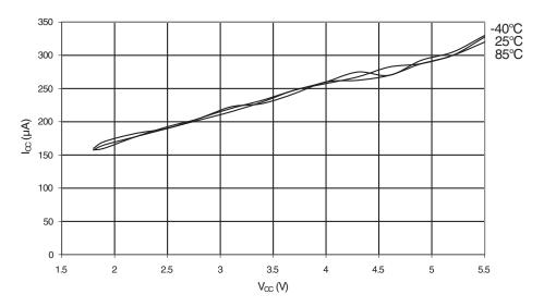
Figure 32-42. AREF External Reference Current vs.  $V_{\rm CC}$
