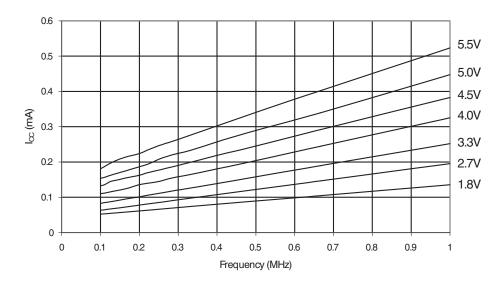
Figure 32-7. Idle Supply Current vs. Frequency (1MHz - 16MHz)
