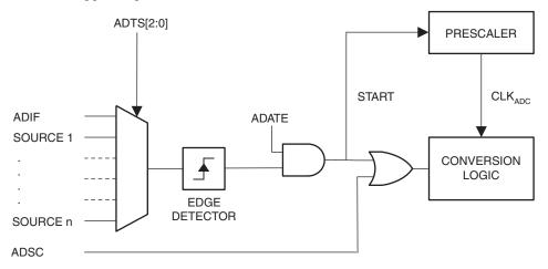
Using the ADC Interrupt Flag as a trigger source makes the ADC start a new conversion as soon as the ongoing conversion has finished. The ADC then operates in Free Running mode, constantly sampling and updating the ADC Data Register. The first conversion must be started by writing a logical one to the ADSC bit in ADCSRA. In
