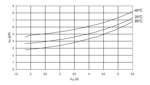
Figure 32-44. Analog Comparator Current vs.  $V_{\rm CC}$
