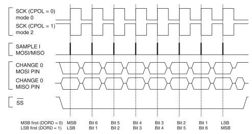
Figure 21-4. SPI Transfer Format with CPHA = 1
