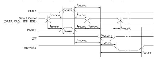
Figure 30-8. Parallel Programming Timing, Loading Sequence with Timing Requirements<sup>(1)</sup>
