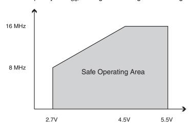
$\textbf{Figure 31-4.} \quad \text{Maximum Frequency vs. V}_{\text{CC}}, \text{ATmega2560/ATmega2561}$
