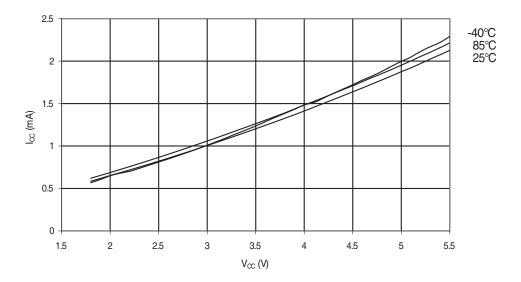
$\textbf{Figure 32-5.} \quad \text{Active Supply Current vs. } V_{\text{CC}} \text{ (Internal RC Oscillator, 128kHz)}$
