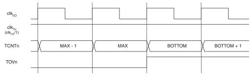
Figure 16-9 shows the same timing data, but with the prescaler enabled.
