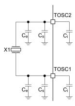
To find suitable load capacitance for a 32.768kHz crystal, consult the crystal datasheet.
