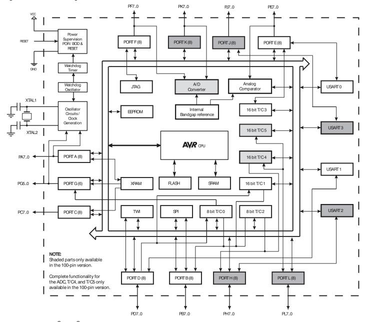
The Atmel® AVR® core combines a rich instruction set with 32 general purpose working registers. All the 32 registers are directly connected to the Arithmetic Logic Unit (ALU), allowing two independent registers to be accessed in one single instruction executed in one clock cycle. The resulting architecture is more code efficient while achieving throughputs up to ten times faster than conventional CISC microcontrollers.
