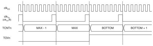
Figure 16-10 shows the setting of OCF0B in all modes and OCF0A in all modes except CTC mode and PWM mode, where OCR0A is TOP.
