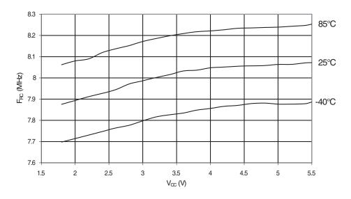
Figure 32-38. Calibrated 8MHz RC Oscillator Frequency vs. Temperature
