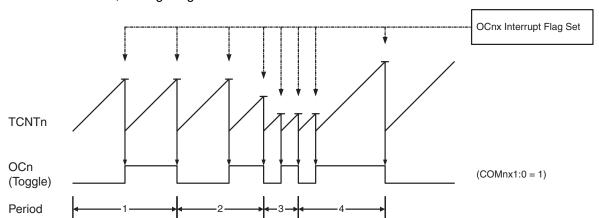
Figure 16-5. CTC Mode, Timing Diagram
