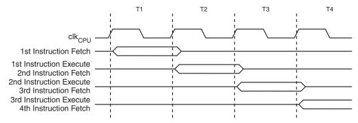
Figure 7-7 shows the internal timing concept for the Register File. In a single clock cycle an ALU operation using two register operands is executed, and the result is stored back to the destination register.
