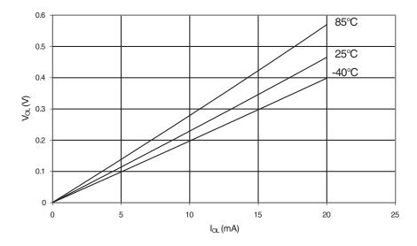
Figure 32-24. I/O Pin Output Voltage vs. Source Current ( $V_{CC} = 3V$ )
