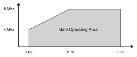
**Figure 31-2.** Maximum Frequency vs. V<sub>CC</sub> when also No-Read-While-Write Section<sup>(1)</sup>, ATmega2560V/ATmega2561V, is used
