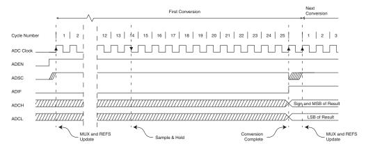
Figure 26-5. ADC Timing Diagram, Single Conversion
