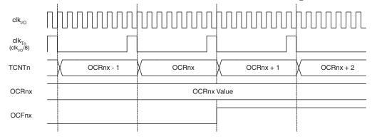
Figure 16-11 on page 125 shows the setting of OCF0A and the clearing of TCNT0 in CTC mode and fast PWM mode where OCR0A is TOP.
