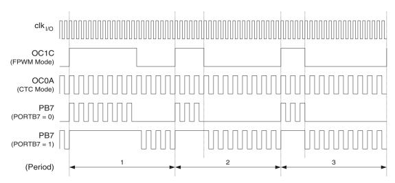
In this example, Timer/Counter2 provides the carrier, while the modulating signal is generated by the Output Compare unit C of the Timer/Counter1.
