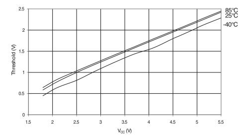
Figure 32-28. I/O Pin Input Hysteresis
