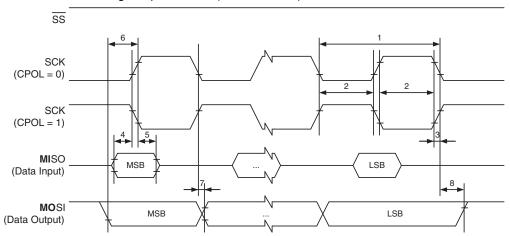
Figure 31-8. SPI Interface Timing Requirements (Slave Mode)
