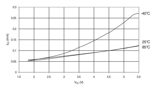
Figure 32-10. Idle Supply Current vs.  $V_{CC}$  (Internal RC Oscillator, 128kHz)I
