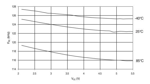
Figure 32-36. Watchdog Oscillator Frequency vs. Temperature
