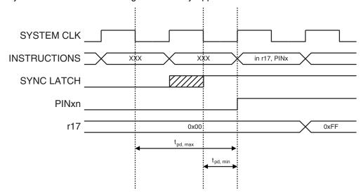
Consider the clock period starting shortly after the first falling edge of the system clock. The latch is closed when the clock is low, and goes transparent when the clock is high, as indicated by the shaded region of the "SYNC"
