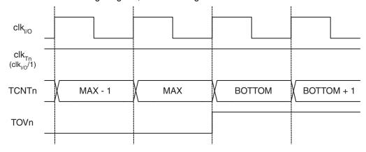
Figure 20-9 shows the same timing data, but with the prescaler enabled.
