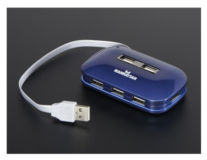
As a bonus you can power the Pi Zero *from* the hub (the power cable does not pass any data) - just plug the power micro USB cable into one of the ports.
