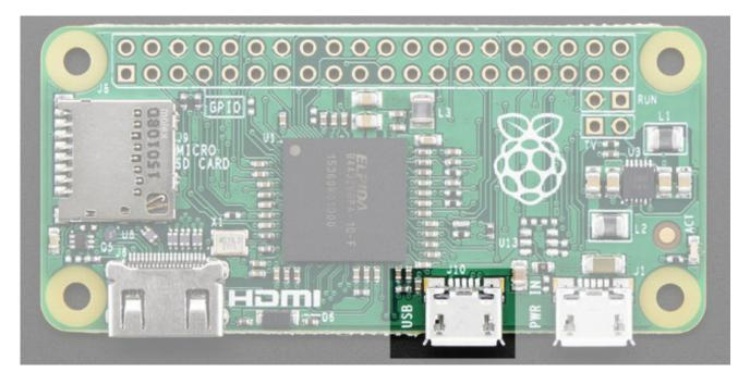
In order to connect a USB device (mouse, keyboard, WiFi) etc you'll need a USB OTG micro B to A cable (http://adafru.it/1099):
