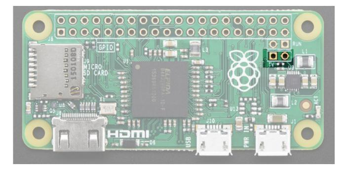
The hole on the left, nearest to the **TV** text, is the signal (+) line, the pin to the right of it is the ground (-) line. Solder two wires to these pads and connect them to an RCA Jack (http://adafru.it/2792) like this one
