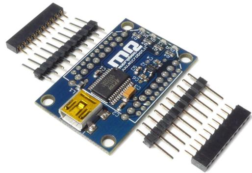
Name: **XBee to USB Adapter**
