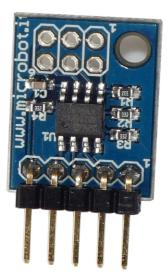
This is a carrier board for the famous Microchip Technology Inc.'s TCN75A digital temperature sensor and it includes all the external components required by the sensor. Its very small size (19x15mm) and its very light weight (only 1.1g), make it the perfect peripheral for small robots and for temperature monitoring systems.
