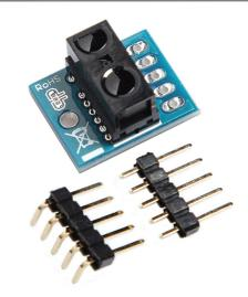
GP2Y0D810Z0F is a distance measuring unit, composed of an integrated combination of PSD (position sensitive detector), IRED (infrared emitting diode) and signal processing circuit.
