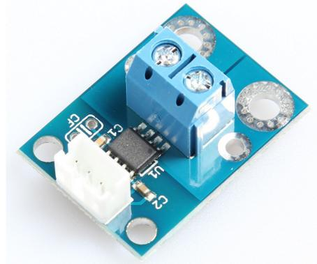
This board carries the Allegro's ACS714ELCTR-05B-T hall effect-based linear current sensor, which offers a low-resistance (~1.2mΩ) current path and electrical isolation up to 2.1kV RMS.
