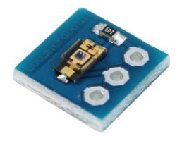
This ambient light sensor carries the TEMT6000 phototransistor. The phototransistor is connected to a pull-down resistor to form a voltage divider that produces an analog voltage output between 0V and +5V as a function of the light detected in the visible spectrum. Lower output voltage is an indication of less light detected.
