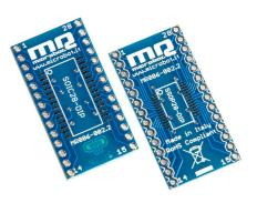
The SSOP28-SOIC28 to DIP Adapter is a double-side board that allows the mounting of 8-28 pin SSOP ICs on one side or the mounting of 8-28 pin SOIC ICs on the other side; in both cases all the signals are broken out through two 0,1" (2,54mm) standard spacing headers that have a 0,6" DIP standard spacing.
