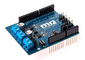
The *Dual DC Motor Shield V2* is a shield that has been projected to enable an Arduino board to drive two brushed DC motors or one 4-wire two-phase stepper motor, controlling the speed and direction of each one independently.
