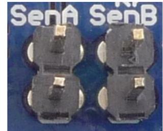
Fig.3 – Jumper del Current sensing
