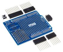
Name: Kit Proto Shield UNO for Arduino
