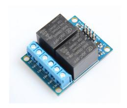
This *Relay Module 2-Channel* is a module designed to allow you to control two relays in a very simple and intuitive manner. Being compatible with Arduino, the most immediate way to use it is to connect it to an Arduino board using flexible jumpers.
