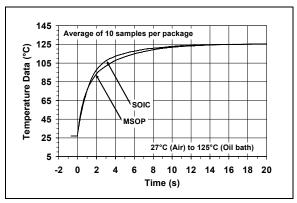
**FIGURE 2-9:** TCN75A Thermal Response vs. Time.
