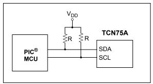
FIGURE 6-1: Pull-up Resistors On Serial Interface.
