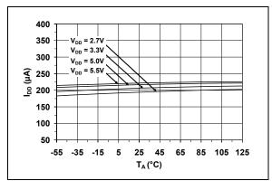
**FIGURE 2-5:** Supply Current vs. Ambient Temperature.
