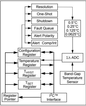
FIGURE 5-1: Functional Block Diagram.
