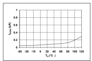
**FIGURE 2-6:** Shutdown Current vs. Ambient Temperature.
