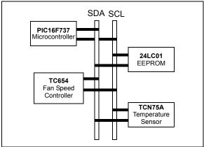
**FIGURE 6-2:** Multiple Devices on I<sup>2</sup>C™ Bus.
